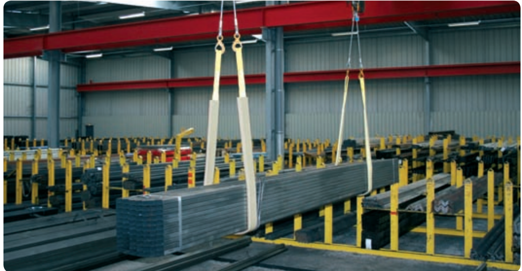
The sliding sleeve enables to reach the right position of the sling without surges.
